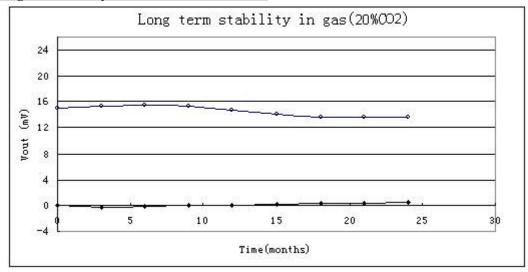
The drift in air is less than 2 mV per year, in 20%CO2 the drift is less than 2mV. for a short period storage (in 2 weeks), the sensor need 30mins' preheating to stabilize, for more than one year storage, it need more than 24 hours' preheating.
